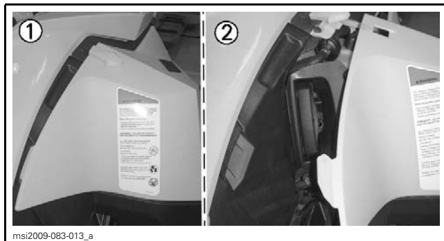
TYPICAL 1. Side panel close 2. Side panel open
